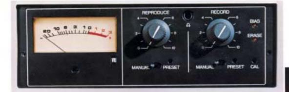
If your application requires more than just the basic ATR-100, then you can add optional input-output modules for a full capability one, two or four-channel recorder. (ATR-101, ATR-102, or ATR-104, respectively.) Each I/O module includes the nor-
